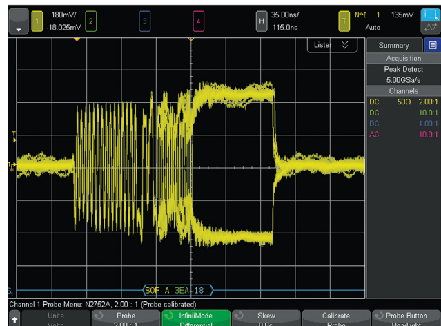
Figure 2: Capturing the hi-speed USB differential signal.
